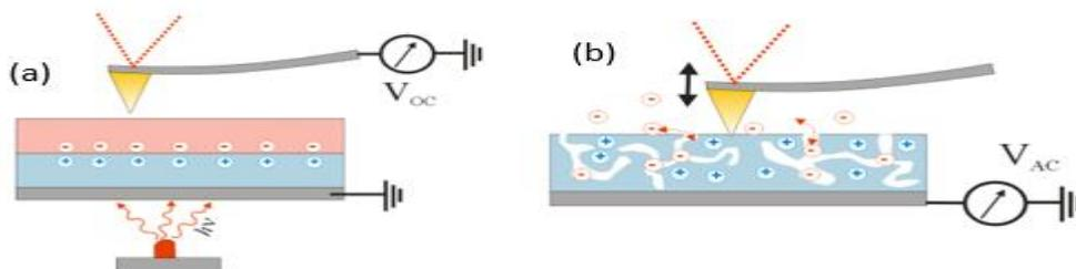
Nanoscale investigation of bioelectronic actuator surfaces: (a) mapping of photovoltage generation; (b) electroswellling due to ion migration.
