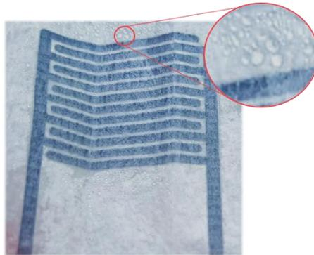
Figure 1: Picture of the PEDOT:PSS sensor printed on the face mask substrate.
