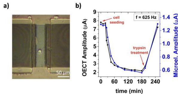
Fig. 2: Single cell detection experiment. a) Microscope image of a single cell placed at the center of a PEDOT:PSS channel with width and length of  $200 \times 50 \mu\text{m}$ , respectively. b) OECT and microelectrode current amplitudes measured at 625 Hz as a function of time. Both sensors are able to measure the cell adhesion after seeding, and recover their original performance after the cell detachment with trypsin.
