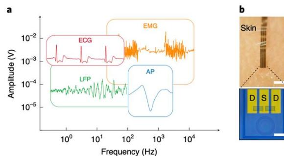
Figure 1: Results reported by Cea et al. in June 2020. (a) Amplitude and frequency characteristics of in-vivo electrical signals. (b) Image of an IG OECT device on human skin (top scale bar = 150  $\mu\text{m}$ , bottom scale bar = 100  $\mu\text{m}$ ). Figure and caption adapted from [5].
