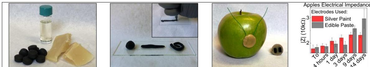
Fig. 1. From left to right. Raw materials that constitute the composite paste: sunflower oil, beeswax, and activated carbon (AC). Pliability of the edible conductor and demonstration of its potential for direct ink writing techniques (inset). Sensor for the detection of aging of apples through impedance measurements. Time-dependent impedance of the apple at 100 kHz recorded with the edible tag (gray column) and using silver paint (red column) as a comparison.
