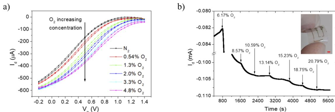
**Figure 1:** a) OECT transfer response upon different dissolved oxygen concentration [0-5% (v/v)] in saline solution. b) Oxygen gas sensing using a flexible, hydrogel-coated OECT in the work-safety range [13-21% (v/v)].
