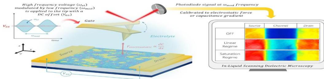
Figure 1: Illustration of In-Liquid Scanning Dielectric Microscopy on Operating EGOFET
