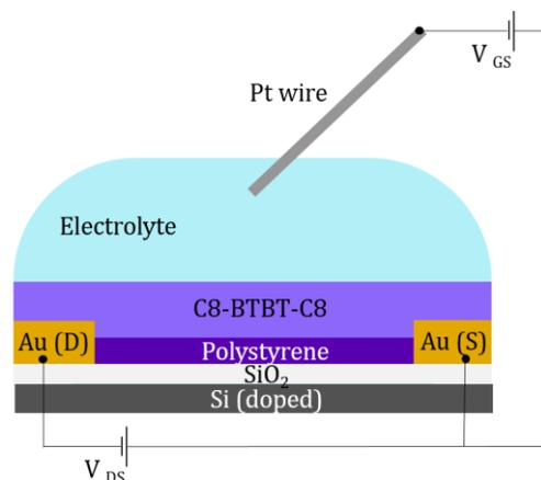
We took electrical measurements in deionized water as electrolyte using both saturation ( $V_{DS} = -0.5$  V) and linear ( $V_{DS} = -0.1$  V) regime to measure transfer characteristics. The best parameters was extracted from the transfer curve in Figure 2:  $V_{th} = 0.03$  V,  $I_{on/off} = 900$ ,  $g_m = 205$   $\mu$ S. To estimate efficiency of the EGOFET we used the following parameter (2):
