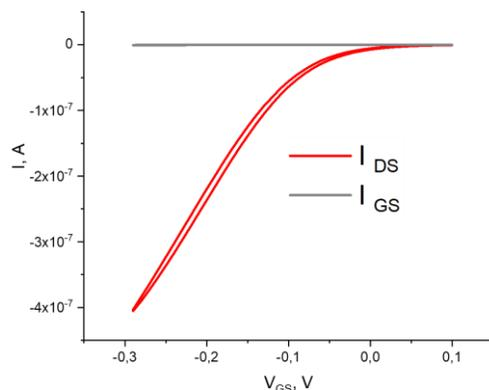
Fig. 2. Transfer characteristics of the EGOFET device recorded at  $V_{DS} = -0.1$  V.
